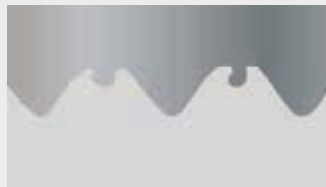
Pre-drilling Ø 17.3 mm
